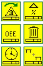
Yellow icons, called “add-ons” are additions to “centers” for optional calculations. These add-ons must be properly glued to the data shapes under the Center. The yellow icons that follow a Center in the Quick stencil can only be used with that Center. Note the first word in the add-on names matches the parent Center.
