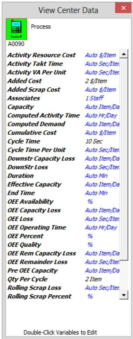
3. Using the “List Variables” form, you can quickly edit any variable by double-clicking on it. For example, the Added Cost for the process was changed the \$2 per item, even though it is a hidden variable.
