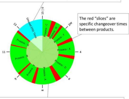
The green "slices" represent production of the different products, eVSM allows for the user to specify the sequence in which production occurs as changeover times between products can vary
